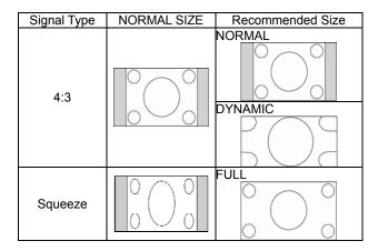
**NORMAL:** Display by the inputted signal aspect ratio by PC signal, or display in 4:3 aspect ratio at DVD/HD or VIDEO signal.
